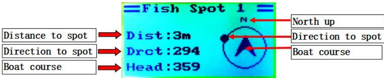
(5) View the real-time distance of the boat from the origin. This function is operated as follows:
