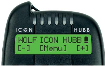
On the HUBB main screen, the HUBB's battery level is displayed. Press and hold the OK button to display the current time and date. [-] [+] Volume settings.
