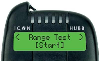
Navigate to the option '**Range Test**' and use the OK button to begin the test. When a connection is established the HUBB will report the signal strength of the connected Alarm and also indicates that the LED is working.
