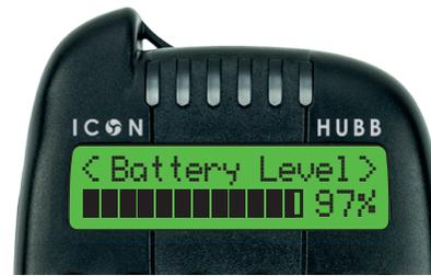
Displays a more precise measurement of the HUBB's battery level. About 500 hrs on Standby.
