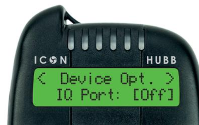
An IQ port accessory that is plugged into to the Alarm IQ Port can be switched On/Off with the HUBB.
