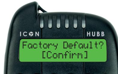
To return the HUBB to factory settings, and clear all user data, power the HUBB off, and then power it back on while holding the
