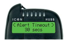
In 'Advanced Menu' Go to 'Alert Timeout' to adjust the time that the LED remains turned on after an alert on the bite Alarm. Press OK and adjust setting using left or right arrows. When confirming this option a message will be sent to the bite Alarm, if successful you will be notified on screen.
