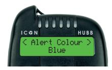
Go to 'Alert Colour' to change the colour used to display alerts on the bite Alarm and HUBB. Press OK and adjust setting using left or right arrows. When confirming this option a message will be sent to the bite Alarm, if successful you will be notified on screen.
