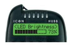
Go to 'LED Brightness' to change the brightness of the LED's displayed on the bite Alarm. Press OK and adjust setting using left or right arrows. When confirming this option a message will be sent to the bite Alarm, if successful you will be notified on screen.
