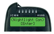
In 'Advanced Menu' go 'Nightlight'. Find the first option titled 'Brightness' and adjust to Manual or Auto setting. Press OK and adjust setting using left or right arrows. When confirming this option a message will be sent to the bite Alarm, if successful you will be notified on screen.
