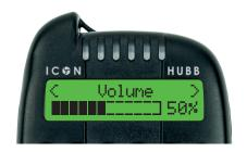
In 'Advanced Menu' go 'Volume' to adjust the volume of the bite Alarm alert. Press OK and adjust setting using left or right arrows. When confirming this option a message will be sent to the bite Alarm, if successful you will be notified on screen.
