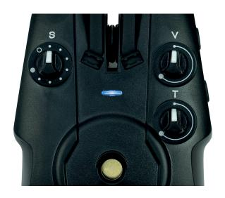
By pressing and holding the someone button the configuration menu can be entered, indicated by the LED's turning white and a special tone. While in the configuration menu the Tone knob adjusts the colour of the Nightlight LED.
