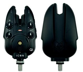
To power up the Bite Alarm, remove the Hard Case and ensure the sensitivity knob is not in the Off position. On start-up the battery level is indicated.
