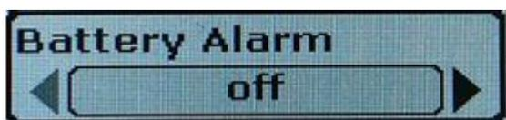
The optional value is Off, 10V to 12V, in increments of 0.1V.
